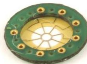
Design - courtesy of Dr. D Moran and M MacEwan, Washington University. Photo above shows a fully assembled device on printed circuit board. Device diameter 6mm.
